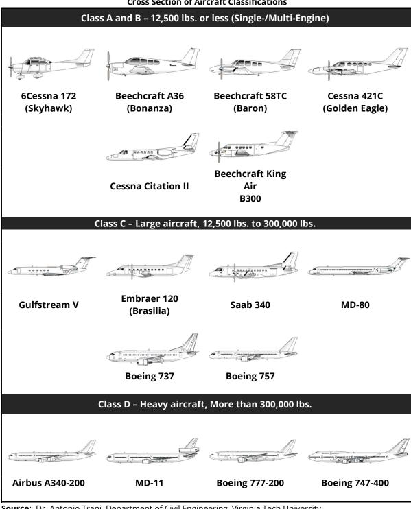
Figure 4-11 **Cross Section of Aircraft Classifications**
